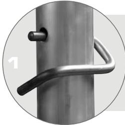
1 All plug-type connections must be secured with gravity pins.
