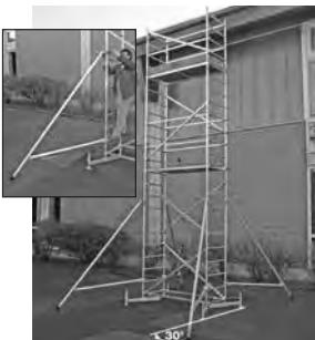
The feet of the outriggers must be placed firmly on the ground. If necessary, use sturdy and altitude equalizing base inserts.
